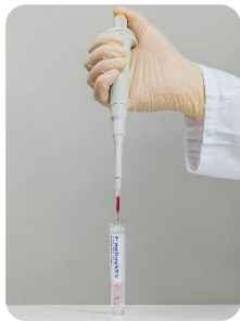
Add your sample liquid to the MTM liquid at a 1:3 ratio
